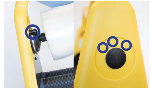
Adjust tension by turning tension knob to the right or left and set into A, B, or C setting. A is highest tension and C is lowest tension setting
