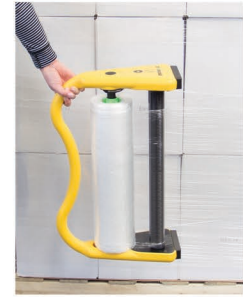
7. Secure end of film to corner of pallet, then pick up Dispenser as shown
